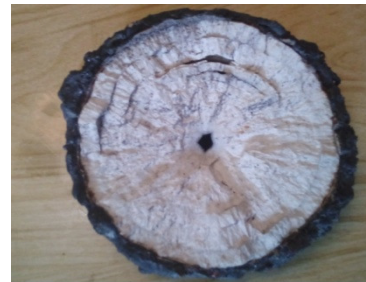
Fig. 8. Pipe section with tsalt deposits before installation of device
